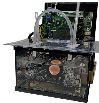
Fig. 3. The modeled two-phase immersion-cooled prototype.
