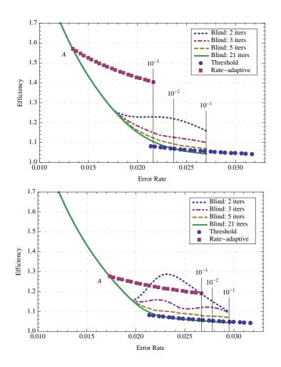
Fig. 6. Estimated efficiency curves, as in Fig. 5, for a coding rate R = 0, 8 and different codeword length,  $2 \times 10^3$  (top) and  $10^4$  (down) bits length. A detailed description is given in text.
