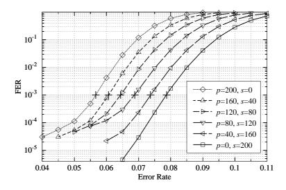
Fig. 3. FER over the BSC for a binary LDPC code of length  $2 \times 10^3$  bits and rate  $R_0 = 1/2$ . Several curves have been simulated for different proportions of punctured and shortened symbols, with d = 200. The distribution of punctured symbols has been chosen according to a pattern previously estimated as proposed in Ref. [23].
