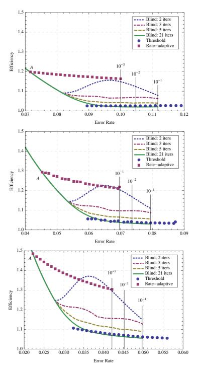
Fig. 5. The estimated efficiency (Gaussian approximation) of the rate adaptive protocol is compared to the efficiency of the blind protocol for short codes  $(2 \times 10^3 \text{ bits length})$ . Three coding rates are used to cover the error range [2.5%, 11%]. A detailed description is given in the text.
