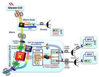
**Fig. 1** Schematics of a possible solution to integrate QKD-links in a classic optical network. The QKD-devices located at the CPE (customer premises equipment) are operated at the O-band and the quantum signals are wavelength-multiplexed with the communication channel.
