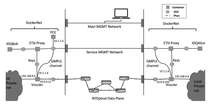
Fig. 6. Logical scheme describing the network used for the end-to-end quantum encryption service via IPsec. The left part shows the DC management and data networks, with a QKD domain (Bob) and a virtual router connected to a PCE. The right part exposes the local network, connecting the other virtual router to the remote PCE and the other QKD domain (Alice). The intermediate area exposes the packet/optical network.
