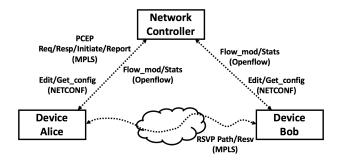
Fig. 2. Generic view of control plane's messages involved in QKD key synchronization process.
